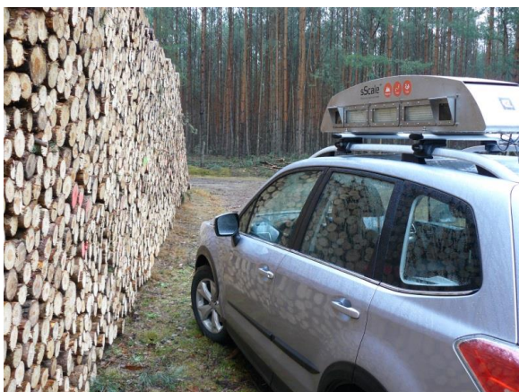
Figure 1: Photo-optical stereo camera system sScale™ 3.4, mounted on the roof rails of a carrier vehicle with two camera units and 3 LED headlamps, in front of an industrial timber stack requiring measurement.
